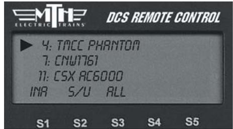
**Note:** The newly added TMCC engine will first appear in the Inactive Engine List. It must be activated by selecting it before the engine will operate.
