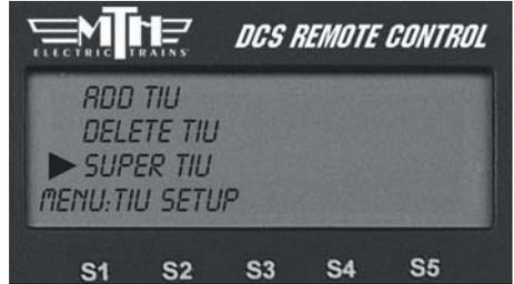
On these multiple TIU layouts, each TIU must have its own, unique TIU address (1 - 5). Each TIU must then be accessed via the remote and changed to a Super TIU. Simply select the Super TIU option under TIU setup for the TIU you are currently editing. Once all the TIUs on the layout have been changed to a Super TIU, an engine can move from section to section of the layout seamlessly.
