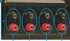
0~22 Volts 10-Volt Track Power (10 AMP) Power (3 AMP) 14-Volt Ac-0~22 Voltscessory PowerTrack Power(3 AMP)(10 AMP)
